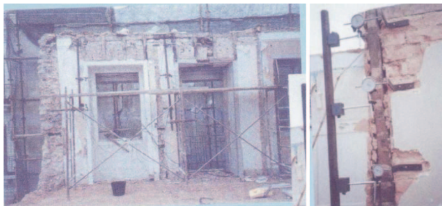
Fig. 9 In-situ tests to rupture [8]
