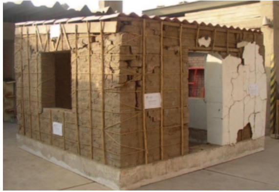
Fig. 28 External cane-rope mesh reinforcement [80]
