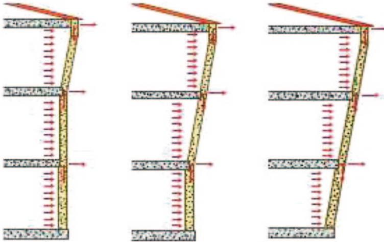
Fig. 18 Out-of-plane failure of façade walls [17]
